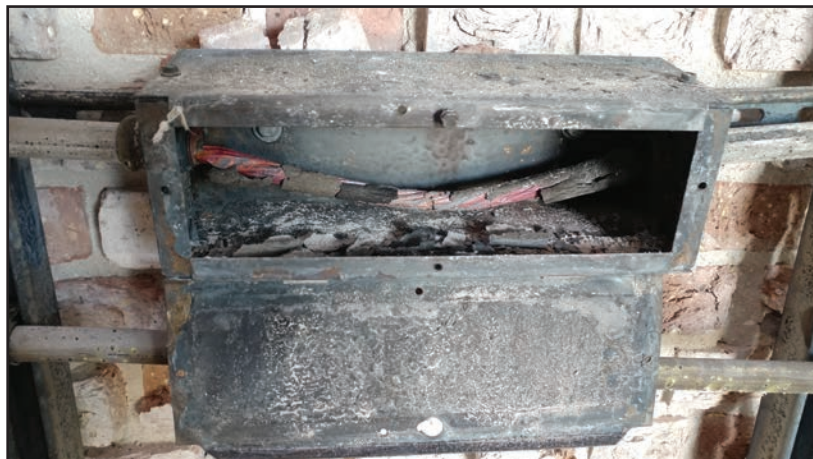
After surviving the extreme heat and hose stream during the 2 hour test, VITALink® cables continue to operate without ever losing signal.
